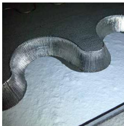
30°坡口 12mm 不锈钢轮廓切割 12 mm Stainless Steel contour with 30° bevel
